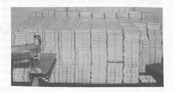
On the next page, the Telex console makes nine C-90 cassettes (both sides) in 6 minutes. The Wollensaks at the bottom right make eight C-90 cassettes in 3 minutes. One person can make over 1,000 a day including handling and labelling.
